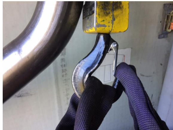
Enactment shows 'Basket Hitch' method used and non-closure of hook
