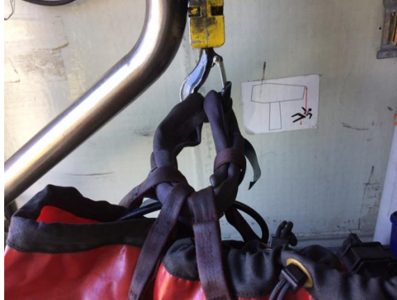
Enactment shows 'Basket Hitch' method and proper closure of hook
