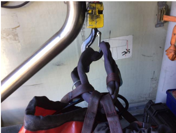
Enactment shows 'Basket Hitch' method used and non-closure of hook
