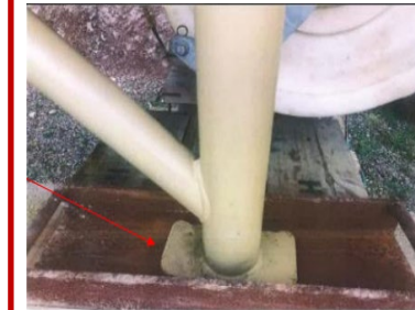
Rubber pads located between the boom foot and the channel section piece of steel.
